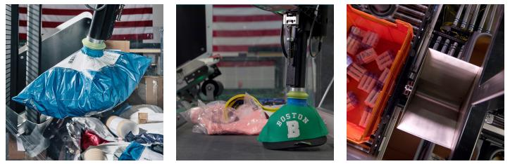
Robotic warehouse systems designed by Berkshire Grey use software, cameras, and sensors to identify individual items and place them in bins or boxes. Vacuum devices are often used to grasp flexible objects such as clothing.
