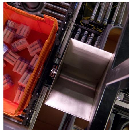
Robotic warehouse systems designed by Berkshire Grey use software, cameras, and sensors to identify individual items and place them in bins or boxes. Vacuum devices are often used to grasp flexible objects such as clothing.
